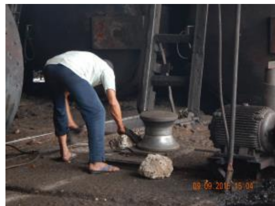
Figure 13. A worker in the mill without PPE
