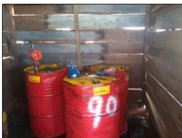
Figure 3 Lubricant store floors are wooden and not sealed.
