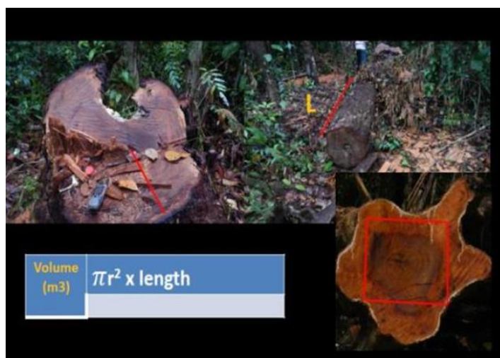
Figure 12. Log cubic measurement. (Source: Proforest)
