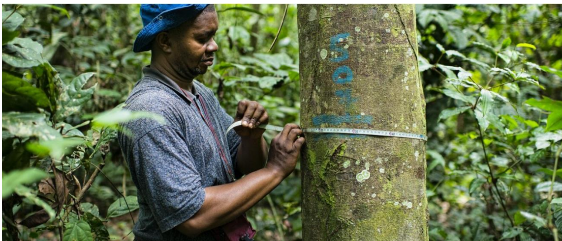
Figure 4. How to measure tree diameter. (Source: Mongabay)
