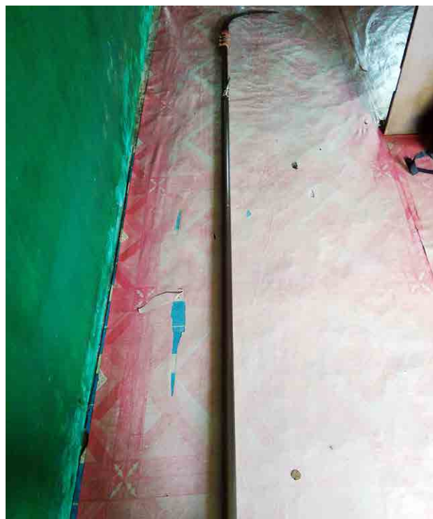
Egrek - long steel poles with a sickle at the end, which can weigh around 12kgs, that harvesters use to cut palm fruit bunches from tall trees. © Private
