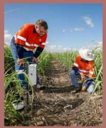
Inspection at a water sampling station to asses the impact of farming practices on runoff water from cane farms
