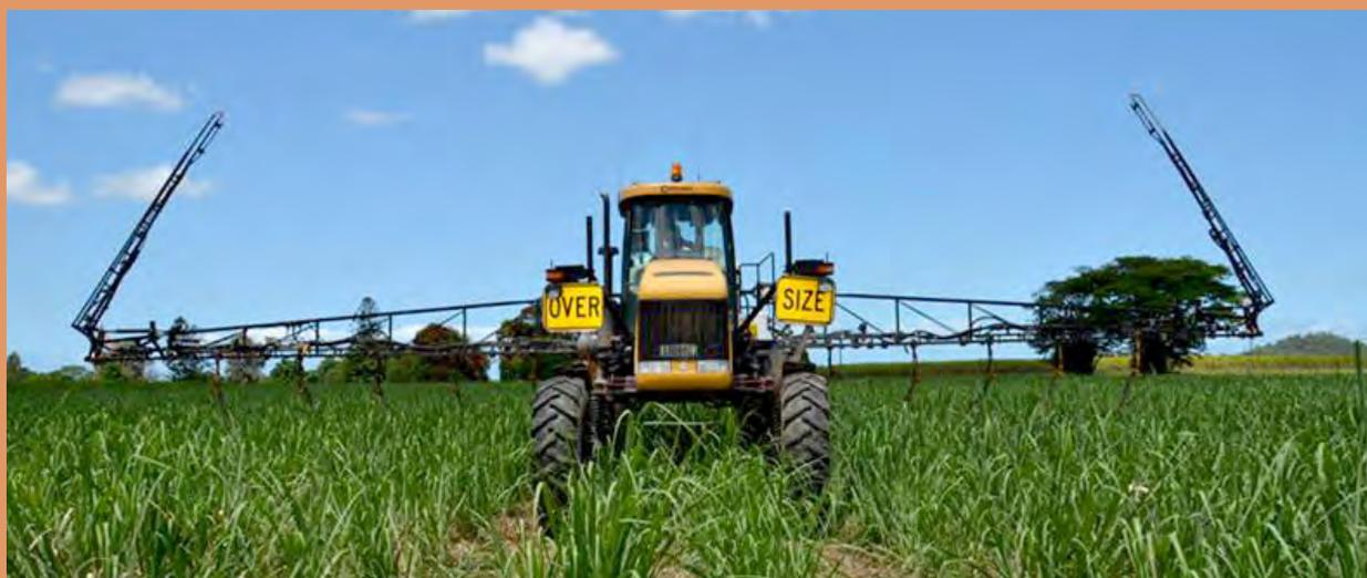
Mechanised spraying of paraquat using booms
